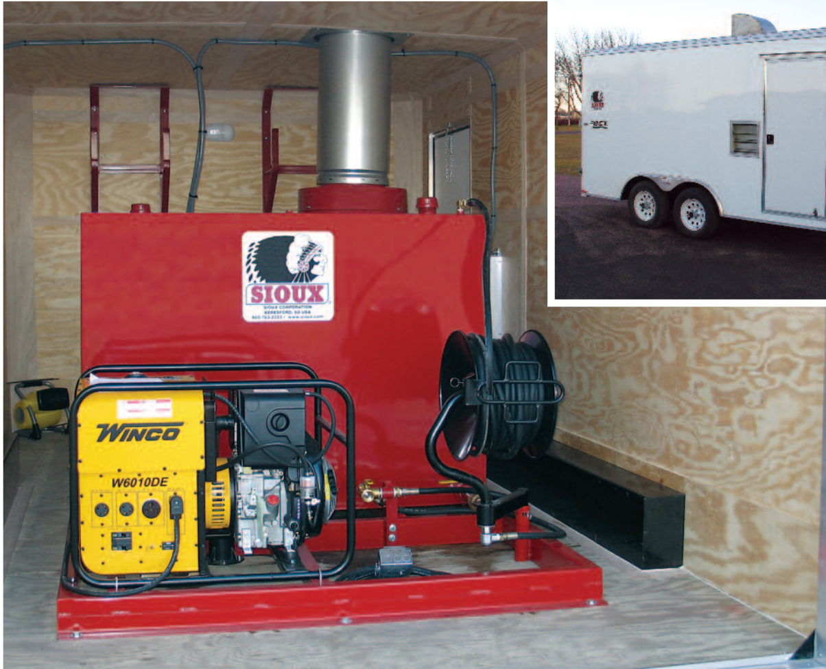
Interior View: SIoux Model S4D250-GTT with insulated trailer
